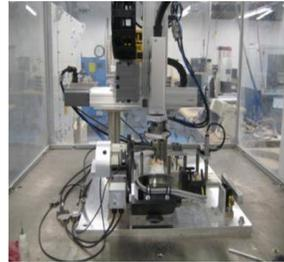
Figure 5: Robocast fabricator
